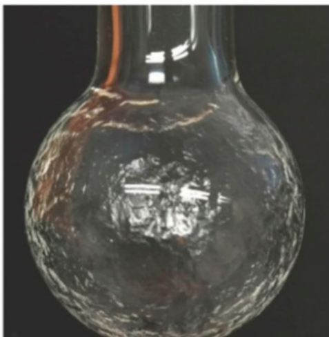
Fig. 1: The eye phantom with RFG gel dosimeter.
