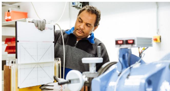
One of two Cobalt calibration benches for calibration and quality control tests of ionization chambers, detectors and detector arrays
