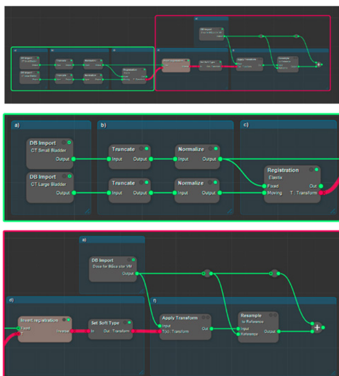
Figure 2. A workflow created in Hero which accumulates the dose given with the planned dose to a patient with two different bladder fillings. The different steps are described below. The upper part shows the entire workflow, with parts zoomed in within the green and red rectangles.
